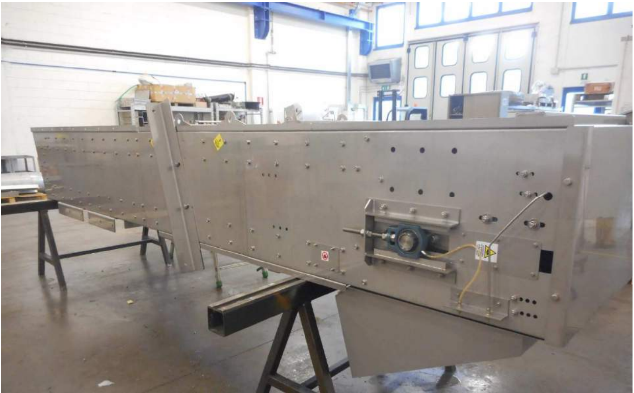
Figure 5 - SMCH multi brushed holed Screen
